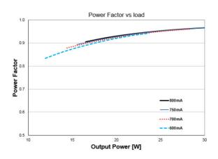
OT FIT 30 CS T Typical Power Factor vs. Load
